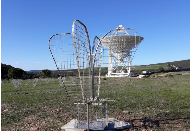
Figure 2. One of the 128 Vivaldi antennas used as front-end of our RFI monitoring system.
