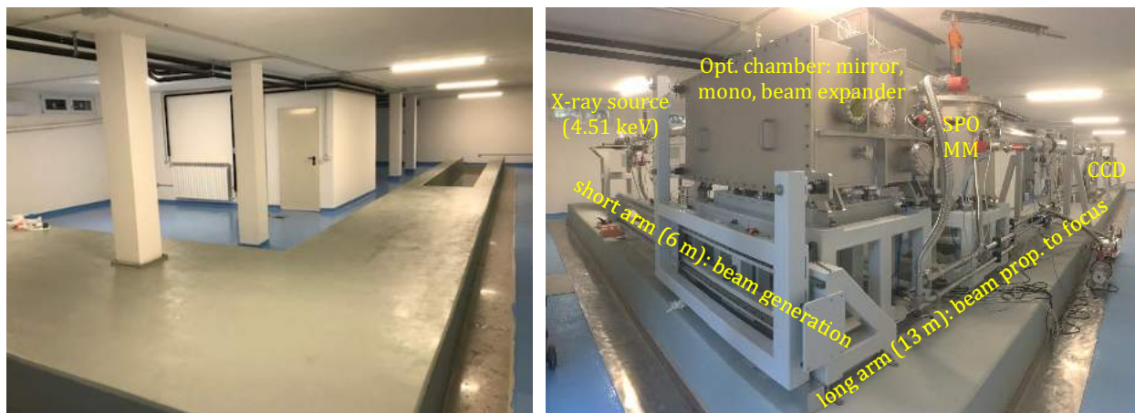
Figure 3: the status of the BEaTriX lab in May 2020 (left) and in July 2021 (right). All the vacuum system was realized and installed by Kenosistec (Binasco, Italy) in a building basement and mounted on an anti-vibration platform. The chambers enclose the optical components that will expand and parallelize the X-ray beam. All the system fits within 17 m × 8 m.
