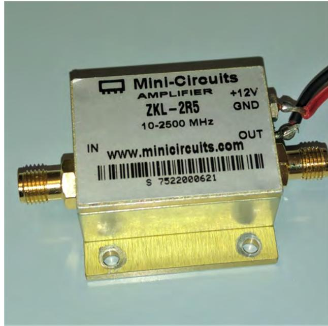
Figura 5: Amplificatore RF MiniCircuits ZKL-2R5, 10-2500 MHz
