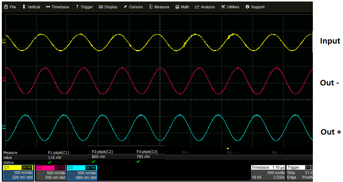
Figure 7. Preamplifier test with an external signal.
