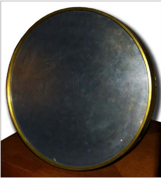
Figure 8: The 20 feet focal length Herschel mirror (photograph: E. Cascone, 2010; courtesy: Astronomical Observatory of Capodimonte).
