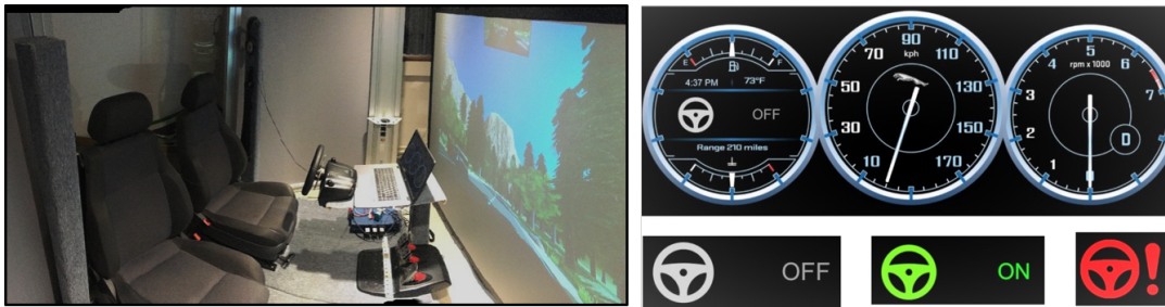
Figure 2: Left: The driving simulator. Right: View of the dashboard and the icons indicating the driving mode.
