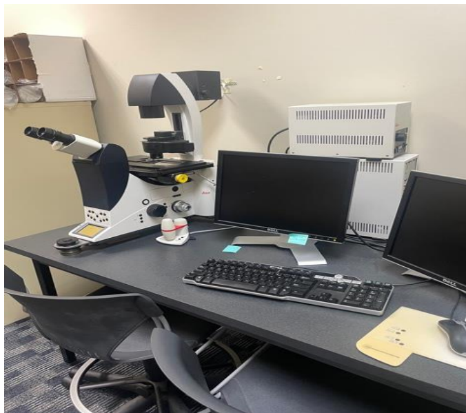
Figure 3-8: Leica DMI 600B Inverted Microscope (Dr. M. DeCoster lab, Louisiana Tech University)
