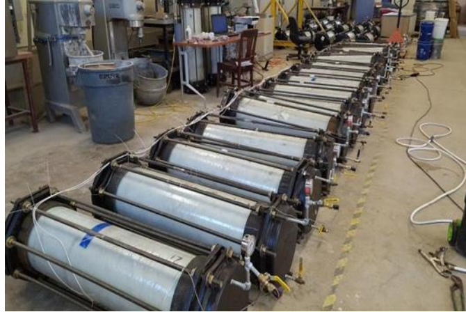
Figure 3-1: Static samples used for ASTM D2992 testing.
