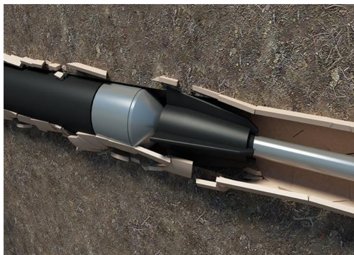
Figure 2-12: Pipe bursting with a modified pulling head – Courtesy of Trenchless Solution
