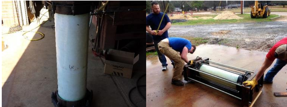
Figure 2-18: Specimen w/MJ caps before attaching threaded rod (left) and liner positioned inside I-beam reinforcement for short term burst (right)
