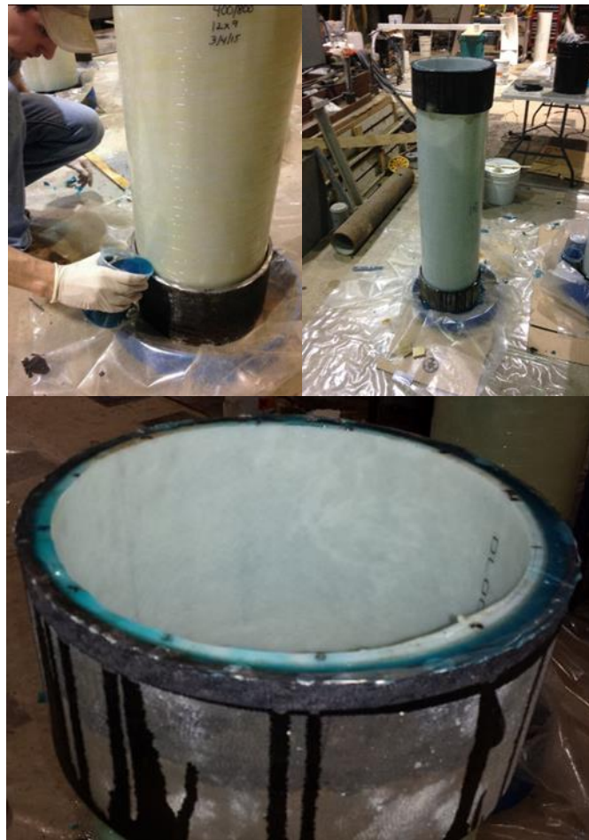
Figure 2-17: Pouring resin in annular space (top left), prepared specimen (top right), and close up of resin after curing (bottom)
