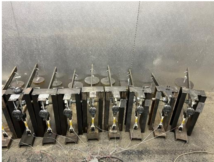
Figure 3-2: Tensile setup commonly used in ASTM D2990 testing.
