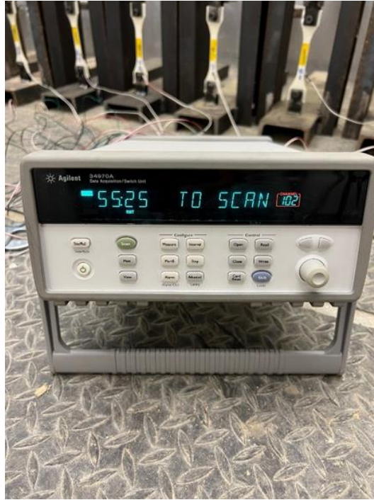
Figure 3-3: Data Logger used for strain data collection.
