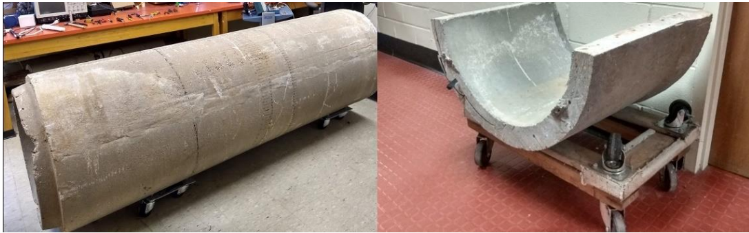
Figure 4-1: Concrete pipe samples.
