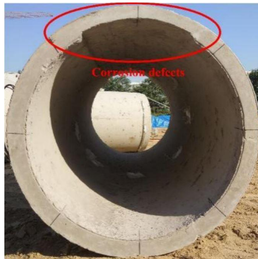
Figure 6-1: Thickness loss due to corrosion [63].
