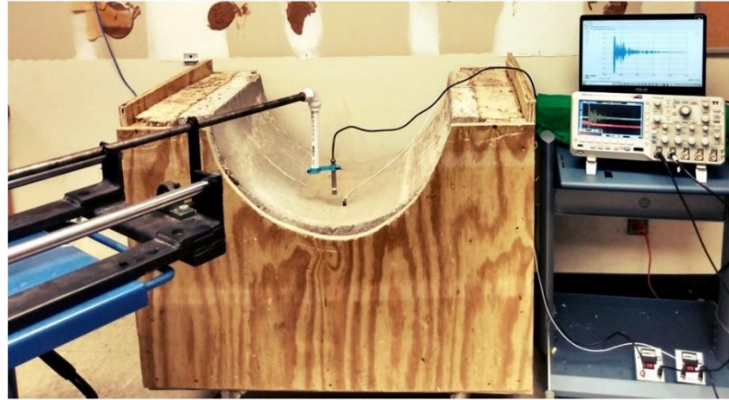
Figure 4-12: Experimental setup for buried concrete pipe.
