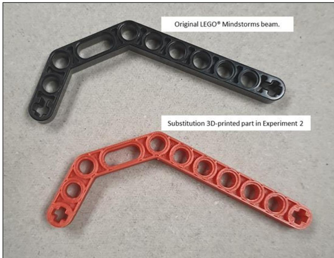
**Figure 6-9:** LEGO double-angled beam (black). The experiment substitution 3D-printed double-angled beam (red).
