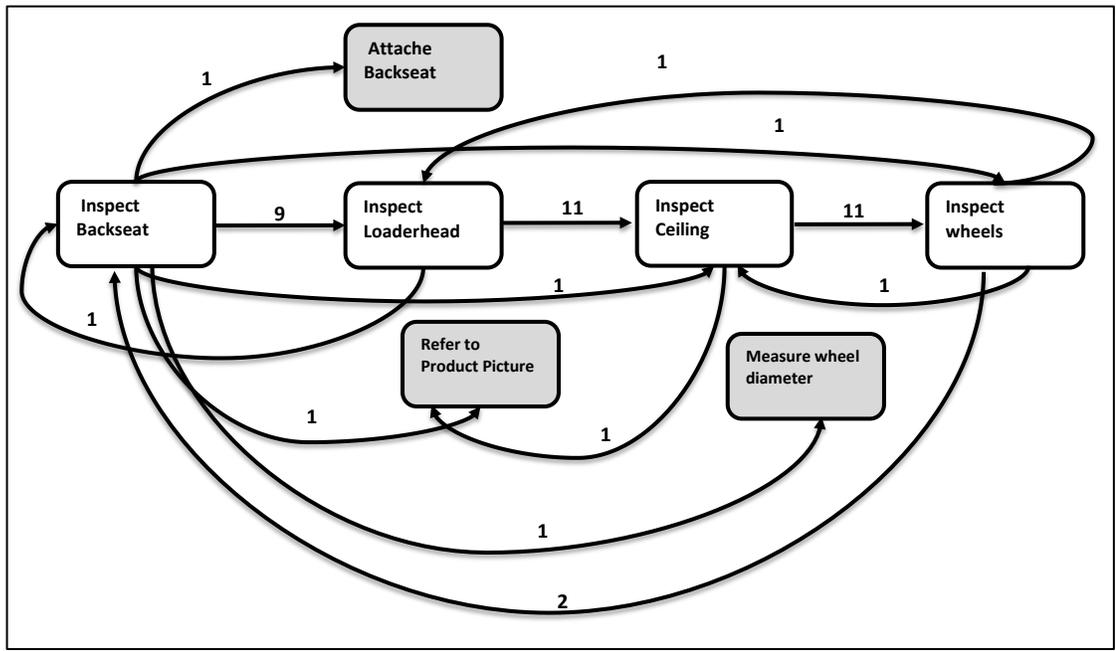
**Figure 5-13:** Actual inspection path the participants followed during the inspection of the toy car assembly.
