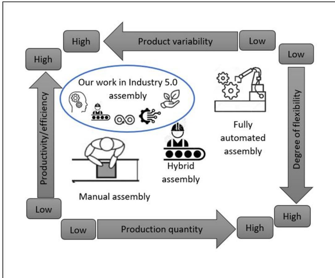
**Figure 6-2:** Manual assembly, hybrid assembly, fully automated assembly, and our research elements in the Industry 5.0 work environment (based on "Changeable and Reconfigurable Assembly Systems by B. Lotter and H.-P. Wiendahl (2009)") [61].
