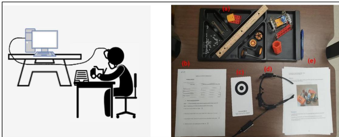
**Figure 4-3:** (Left) Single workstation configuration with seated worker. (Right) The workbench layout with (a) toolbox (b) measurements and inspection sheet (c) calibration target (d) eye-tracking glasses (e) assembly instructions sheet.
