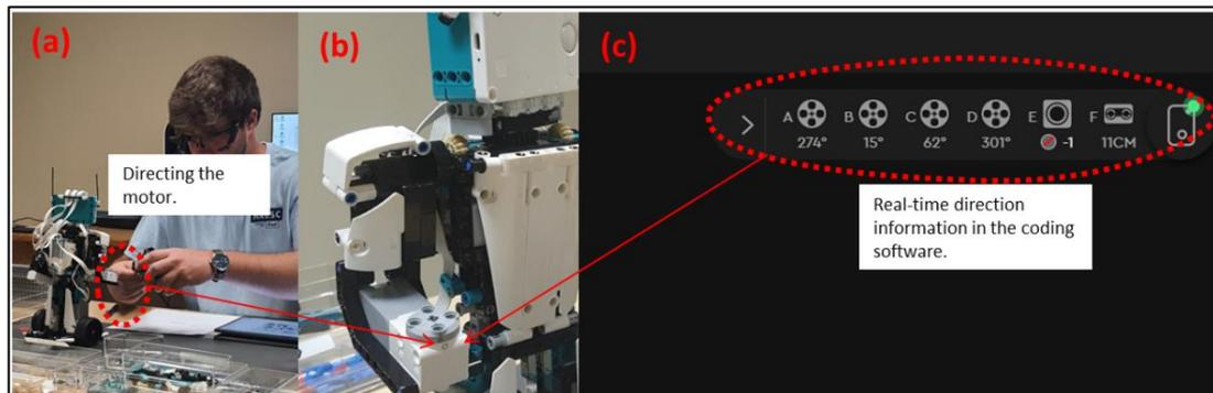
**Figure 6-7:** Manual assembly of the robot's claw. (a) Assembler directing the motor in the specified degrees. (b) Enlarged view of the arm's motor in the zero direction. (c) Real-time positioning data which the assembler monitors simultaneously in Mindstorms® software.
