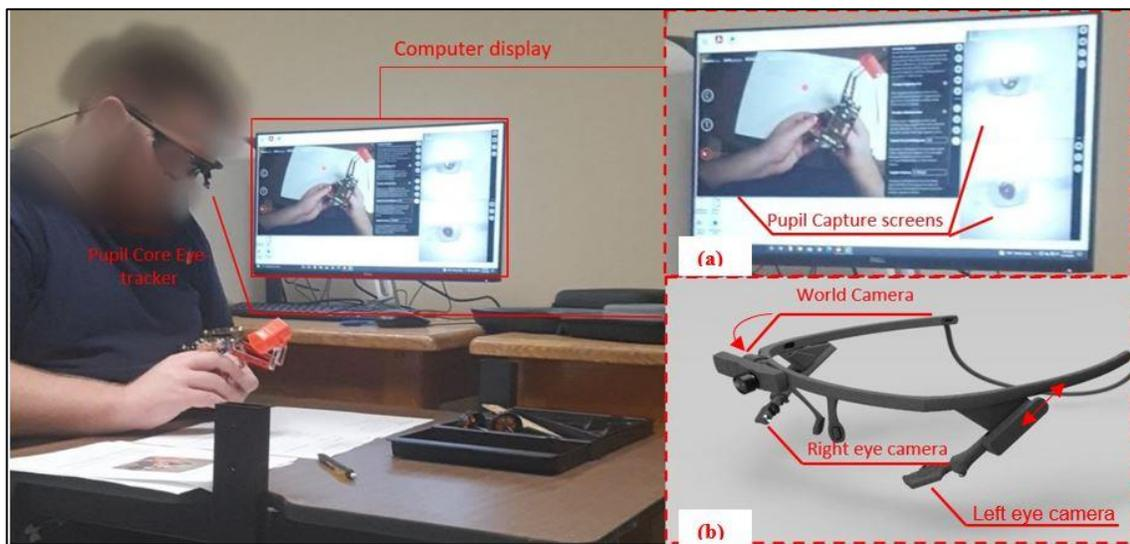
**Figure 4-1:** (Left) Experimental apparatus. (Right) (a) Pupil Capture desktop app real-time display of the experiment captured by the eye tracker cameras (b) Pupil Core eye tracker.
