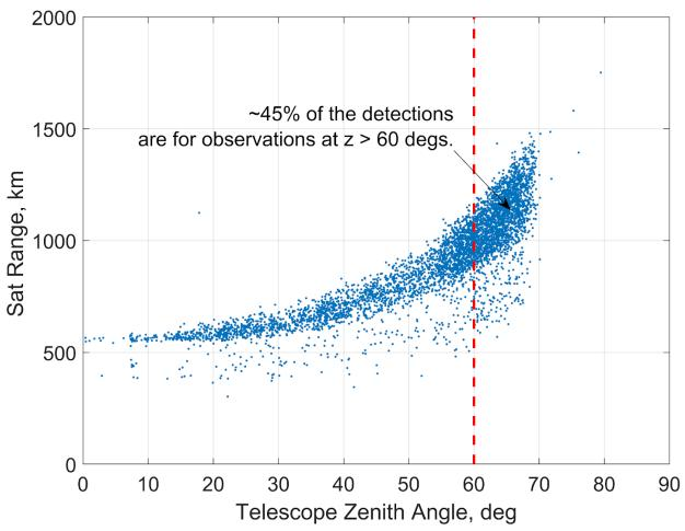
Figure 5.5. Scatter plot of the satellite streaks detected in the ZTF images as a function of telescope zenith angle and satellite range.
