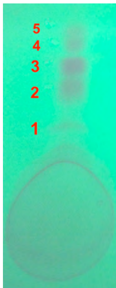
Figure 1: Compound separation of the methanol extract of N. lobata under UV detection (254 nm). All replicates of this material under the given conditions yielded five distinct spots.
