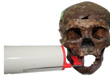
Figure 8. The position of the holder testing against the cadaveric skull
