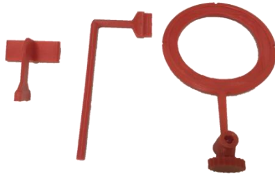
Figure 5. The result of printing the holder using a 3D printer
