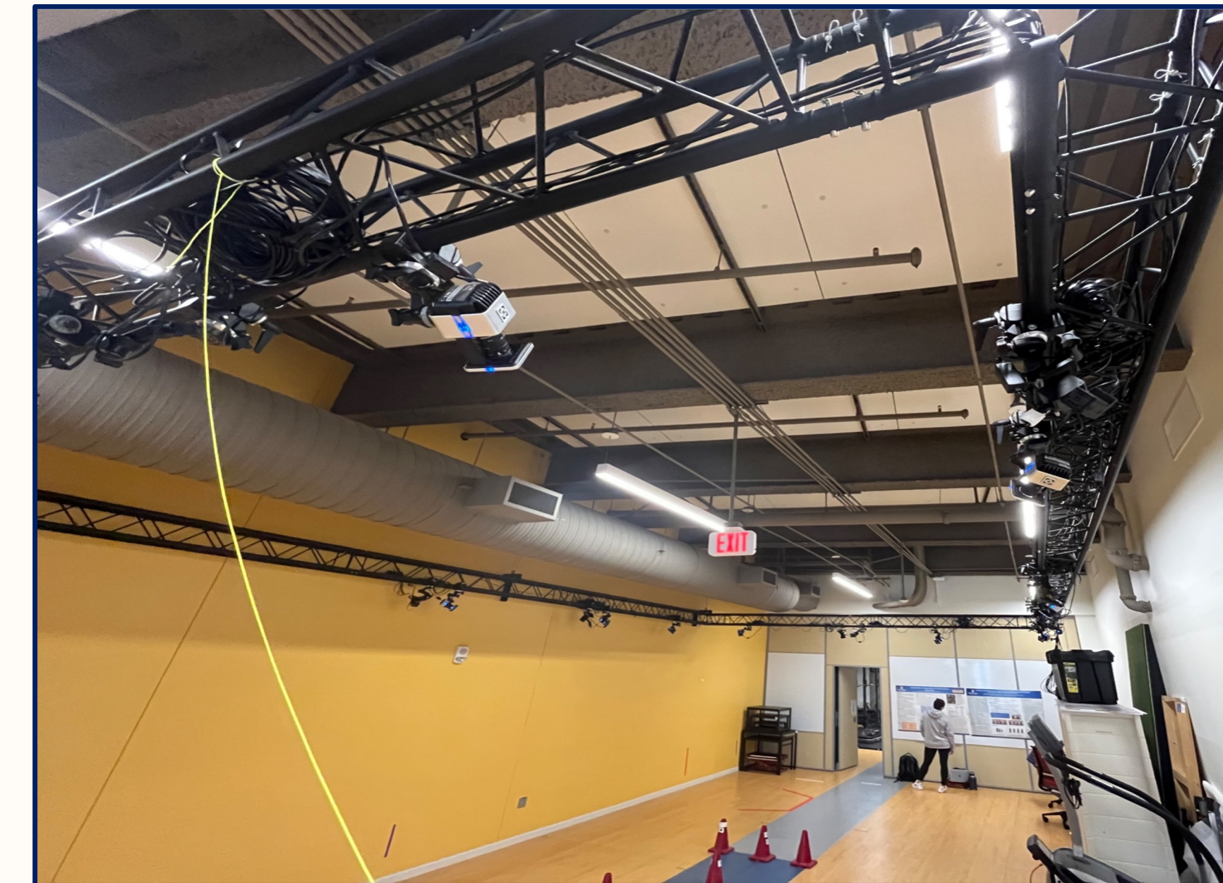
Figure 2. The Theia Markerless Measurement System, used to measure segment lengths
