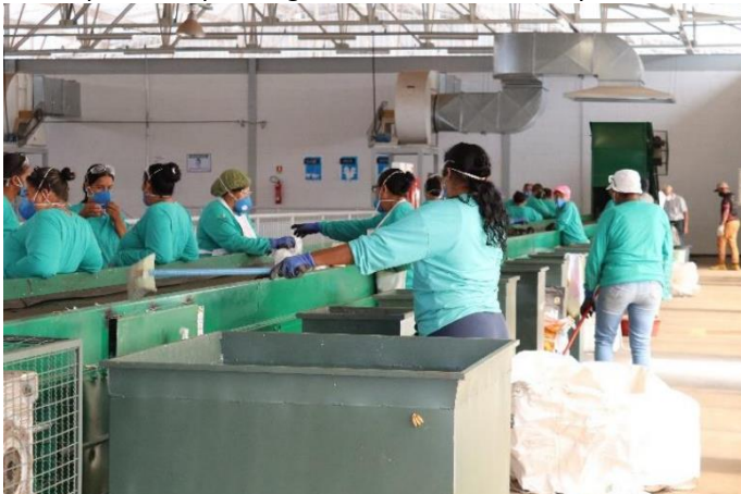
Figure 1 Waste pickers separating materials on the conveyor
