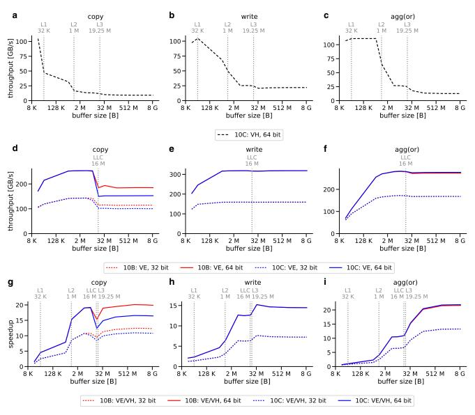
Fig. 6 Single-thread sequential memory access evaluation: measured throughput of VH and VE as well as the speedup obtained by the VE of different IO-operations executed using one thread
