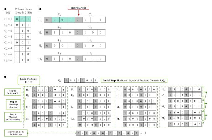
Fig. 4 Illustration of BitWeaving/H [27]. a Data, b BitWeaving/H, c Predicate Evaluation
