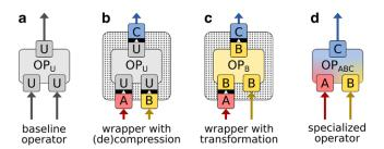
Fig. 3 Integration of compression and operators. A to C are compressed formats; U is uncompressed [7]
