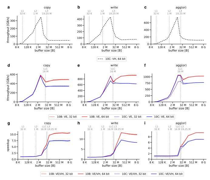
Fig. 9 Multi-thread sequential memory access evaluation: measured throughput of different IO-operations executed on the VH using multiple threads
