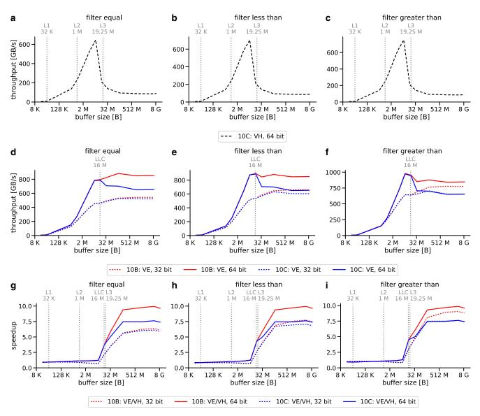
Fig. 10 Multi-thread column scan evaluation: measured throughput of different Bitweaving-H operations executed on the VH and the VE using multiple threads
