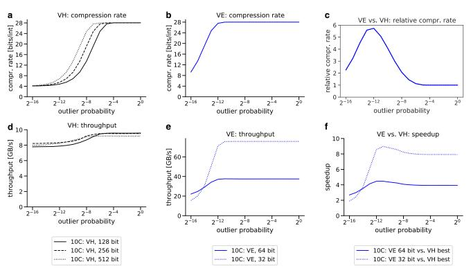
Fig. 7 Single-thread BP compression evaluation: measured compression rate of BP on VH and VE for different outlier probabilities
