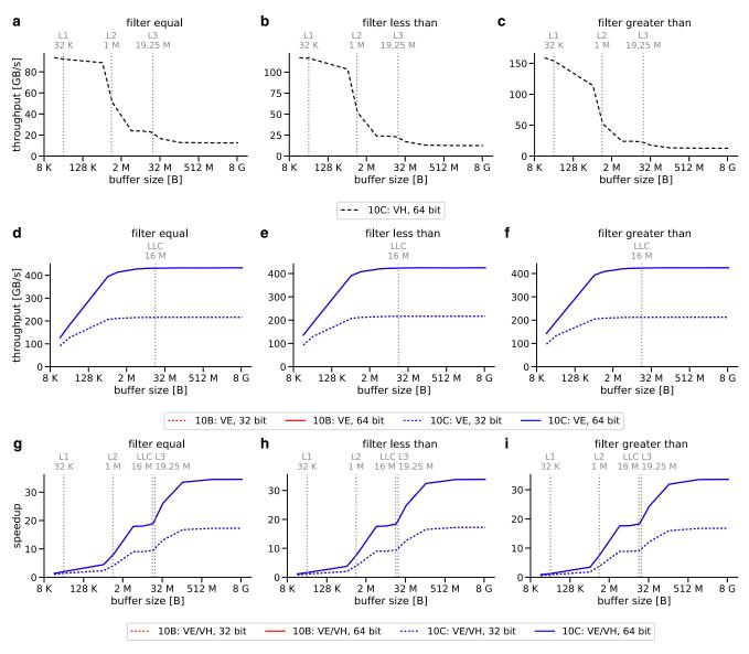
Fig. 8 Single-thread column scan evaluation: measured throughput of VH and VE as well as the speedup obtained by the VE of different BitWeaving/H-operations executed using one thread
