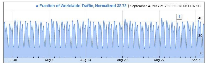
Fig. 1: The normalised traffic of Google Search for Germany. The normalised traffic is obtained by computing the ratio of Germany’s request rate to the worldwide request rate, resulting in a number between 0 and 1. Then Google multiplies the number by a constant, which normalises but does not change the shape of the graph. The same approach was adopted in Fig. 2.
