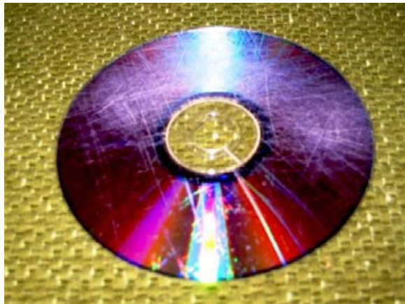
Figure 3: Severely damaged DVD disk
