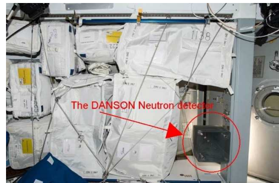
Figure 2. The DANSON detector payload location, labelled SND (top) in the payload topology forum rendering for the International Space Station (ISS) Node 2 Zenith. At the bottom, the actual detector cube is shown affixed to the light bridge structure running between the starboard and overhead hatches on the zenith side of ISS Node 2 (Harmony) module of the ISS. Its facing was to the overhead (zenith) hatch. It was surrounded on three sides by cargo stowage bags filled with crew laundry and the on the fourth side by the Columbus module.
