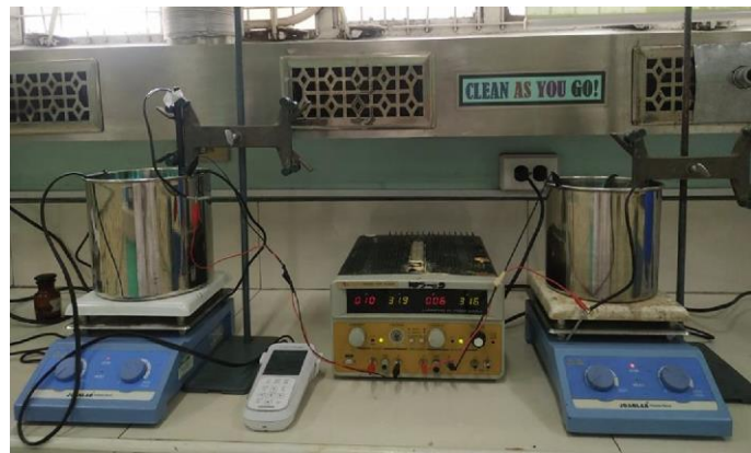
Fig. 1 - Self-fabricated photoelectron Fenton process composed of steel cylindrical reactor, voltage source, hotplate, anode and cathode terminals and pH meter
