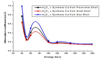
Fig. 9 - Linear attenuation coefficient against energy for the composites
