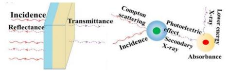
Fig. 1 - Attenuation mechanisms of x-ray [7]
