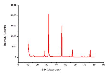
Fig. 4 - X-ray diffraction of the synthesized Al<sub>2</sub>O<sub>3</sub> Powder
