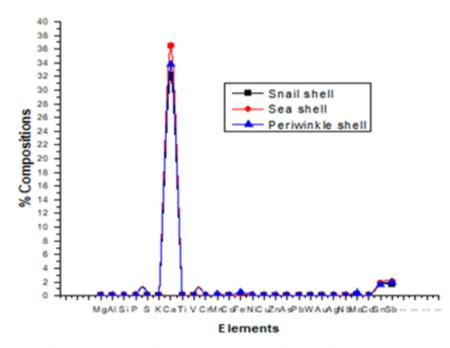
Fig. 5 - XRF analyses of the calcined samples from different shells particles
