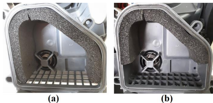
Fig. 3 - (a) 100% coated inner wall; (b) 70% coated inner wall with K-flex K-FONIK open cell
