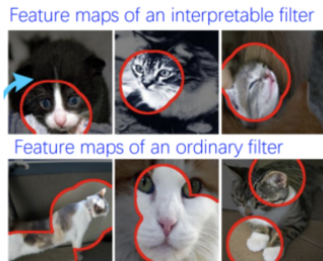
Figure 3: The top CNN filter clearly identifies the cat's face as the rationale for detecting a cat. The bottom CNN filter has a less clear identification strategy, akin to F1 and F2. 20
