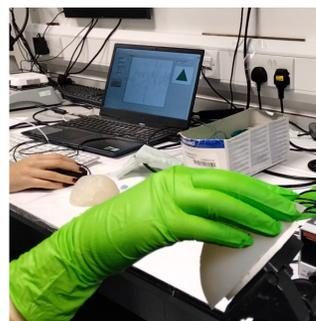
Fig. 3. Pilot study setup, with the participant using the sensor glove on the phantom fetal head
