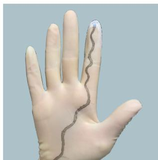
Fig. 1. The sensor glove, used to detect sutures
