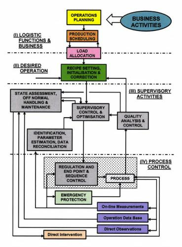
Figure 6.2: Functions for Operations of Process Plants
