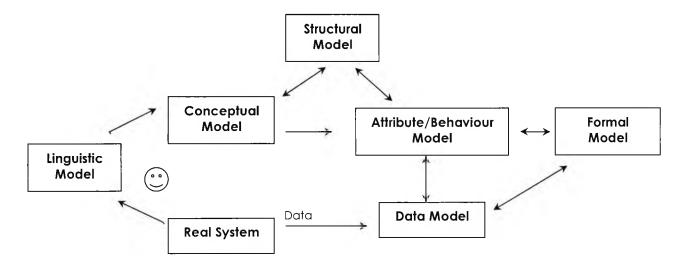
Figure 5.3: Relations between different stages of modeling
