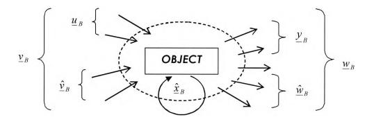
Figure 3.3: Embedding of an Object and Classification of Variables
