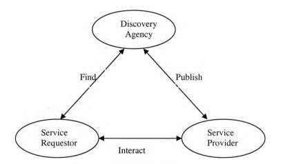
Figure 2.1: Basic web-service architecture
