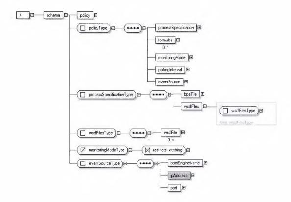
Figure 3.1: Graphical view of the monitoring policy schema
