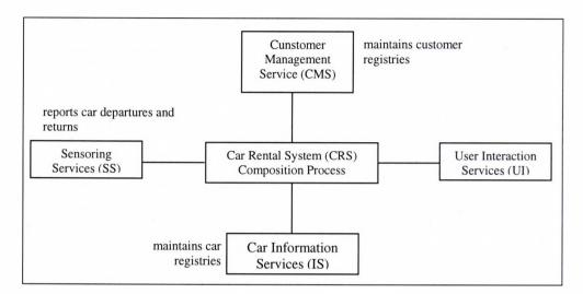
Figure 4.1: Structure of the car rental system (CRS)
