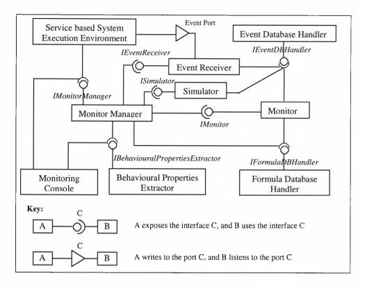
Figure 5.1: Implementation architecture of the monitoring framework
