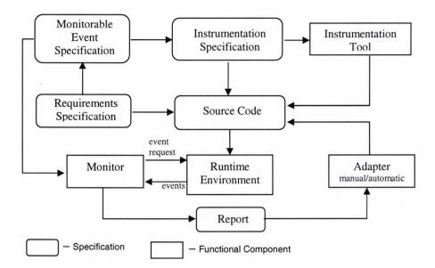
Figure 2.14: A general framework for requirements monitoring
