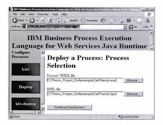
Select the WSDL and BPEL file of the process to be deployed, then click on the "Continue Deployment" button. A new page will appear as shown below. In the new page select WSDL files (only one in this example) for all the services deployed by the BPEL process. Click on the "Start Serving the Process" button. A new page will appear to confirm the successful deployment of the process.
