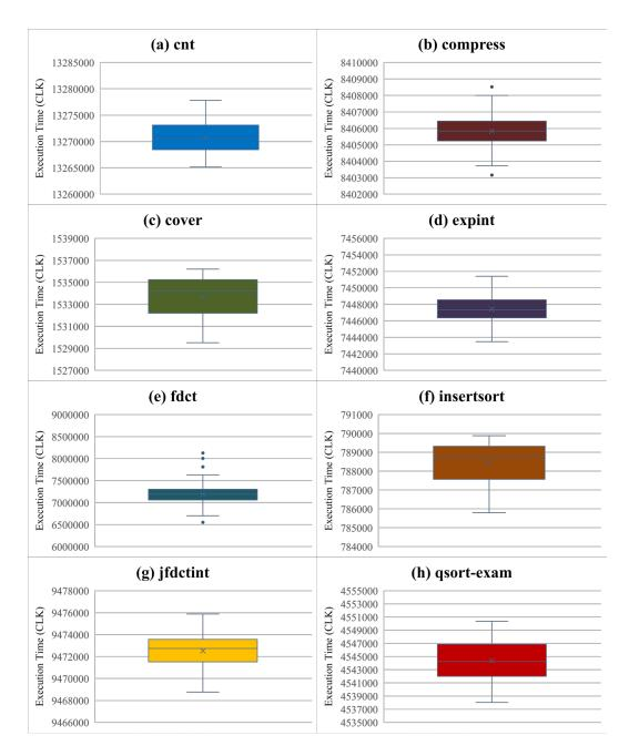
Figure 6.13. Boxplot of Execution Time in  $8 \times 2$  Meshed Bluetree Architecture with Instruction DRAM Module and Data DRAM Module
