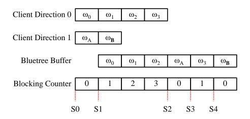
Figure 4.3. Blocking Behaviour of Bluetree Multiplexer
