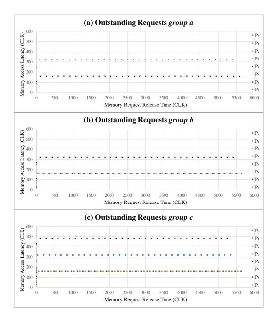
Figure 4.6. Memory Access Latency across 8-Client TDM Tree-based Architecture
