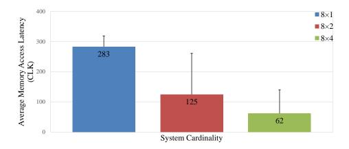
Figure 6.9. Average Memory Access Latency with Multiple Homogeneous Memory Modules
