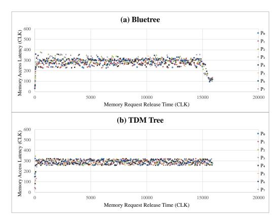
Figure 4.7. Memory Access Latency with Balanced Path Workloads across 8-Client Bluetree-based Architecture and 8-client TDM Tree-based Architecture
