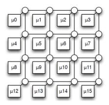
Figure 1.1. Network-on-Chip Architecture
