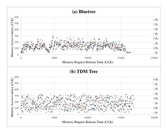
Figure 4.9. Memory Access Latency with Increasing Request Intervals across 8-Client Bluetree-based Architecture and 8-client TDM Tree-based Architecture
