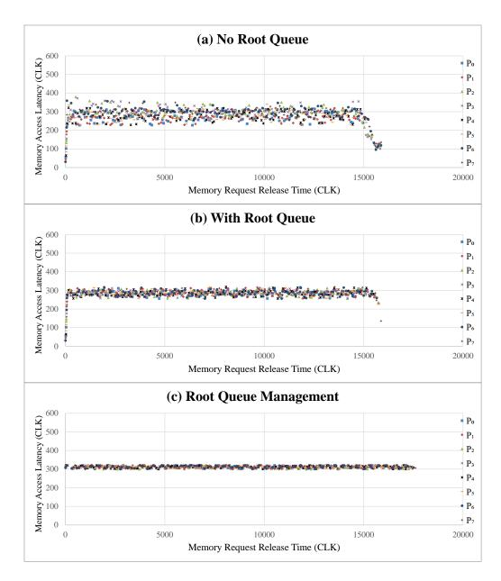
Figure 5.8. Memory Access Latency with Balanced Path Workloads
