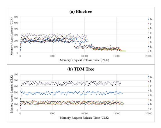
Figure 4.11. Memory Access Latency with Unbalanced Path Workloads across 8-Client Bluetree-based Architecture and 8-client TDM Tree-based Architecture
