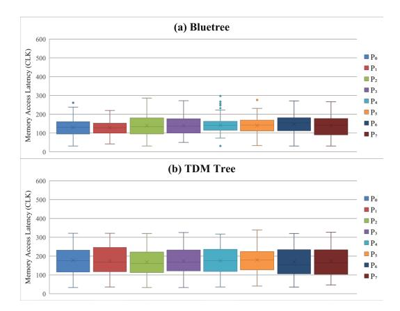
Figure 4.10. Boxplot of Memory Access Latency with Increasing Request Intervals across 8-Client Bluetree-based Architecture and 8-client TDM Treebased Architecture
