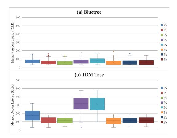
Figure 4.14. Boxplot of Memory Access Latency with Varying Request Intervals across 8-Client Bluetree-based Architecture and 8-client TDM Tree-based Architecture
