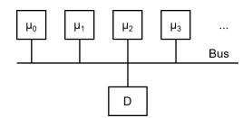
Figure 2.9. Bus-based Multi-Core Architecture
