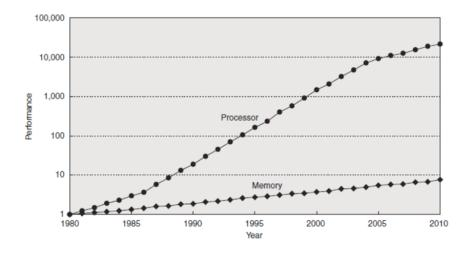
Figure 1.2. Performance Gap between Memory and Processor [10]
