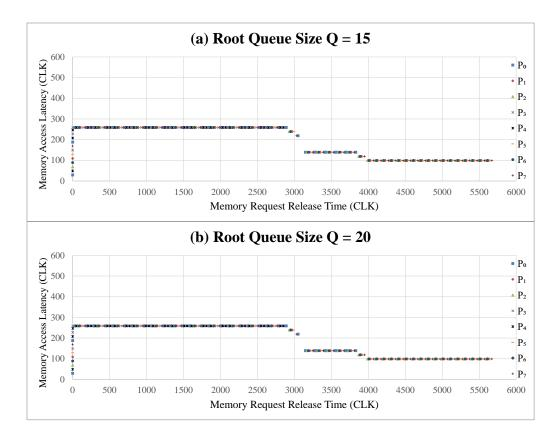
Figure 5.5. Memory Access Latency with Increased Root Queue Size
