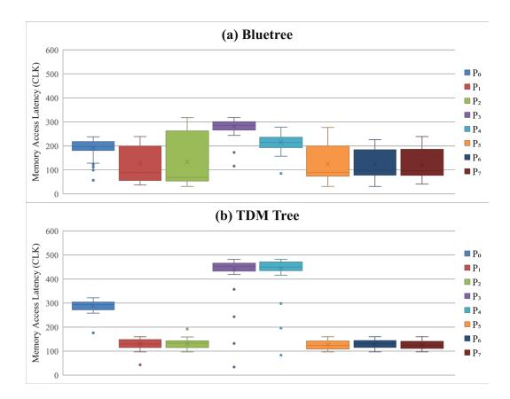
Figure 4.12. Boxplot of Memory Access Latency with Unbalanced Path Workloads across 8-Client Bluetree-based Architecture and 8-client TDM Treebased Architecture
