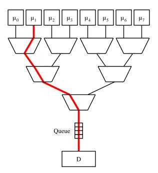
Figure 5.2. Bluetree-based Architecture with Root Queue Modification
