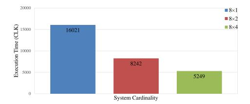
Figure 6.8. Execution Time with Multiple Homogeneous Memory Modules
