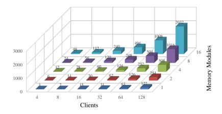
Figure 6.5. Hardware Consumption: Bluetree Multiplexer
