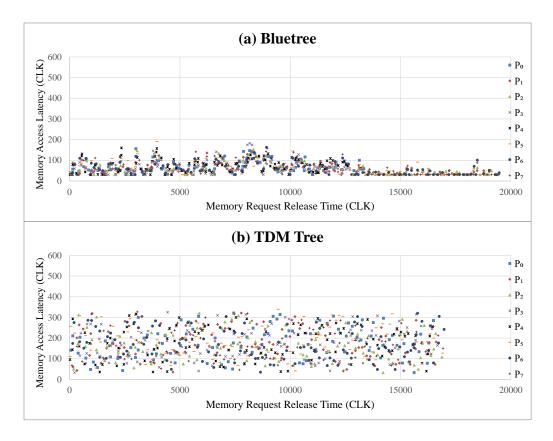
Figure 4.13. Memory Access Latency with Varying Request Intervals across 8-Client Bluetree-based Architecture and 8-client TDM Tree-based Architecture
