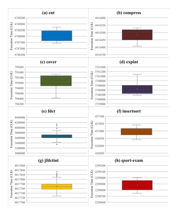
Figure 6.14. Boxplot of Execution Time in  $8 \times 2$  Meshed Bluetree Architecture with Dual DRAM Modules
