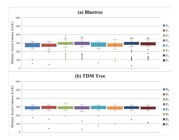
Figure 4.8. Boxplot of Memory Access Latency with Balanced Path Workloads across 8-Client Bluetree-based Architecture and 8-client TDM Treebased Architecture
