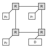
Figure 2.11. Shared Memory Network-on-Chip Architetcure
