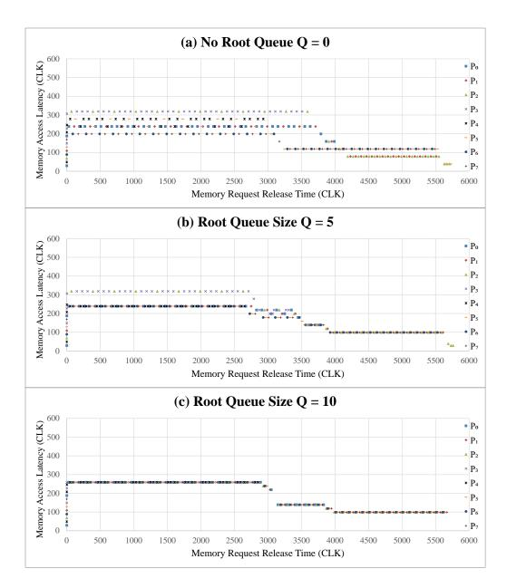
Figure 5.4. Memory Access Latency with Increasing Root Queue Size
