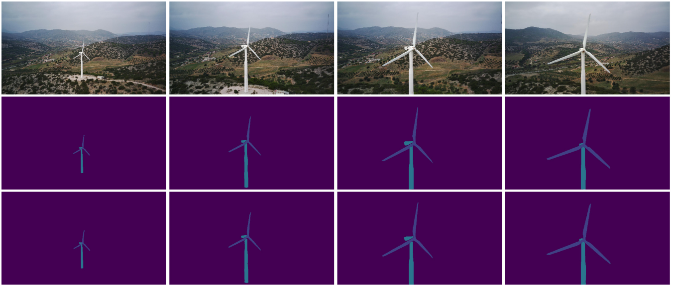
Fig. 9. WTA Wind turbine navigation scenario: The UAV detects a wind turbine target and moves closer to it. Top row contains RGB images, middle row contains ground truth data and bottom row contains DDRNet23-slim-hix2 segmentation maps.
