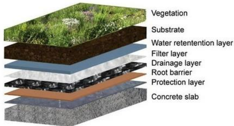
Figure 1.4: A schematic of the layers in an example green roof (Brachet et al. 2019)
