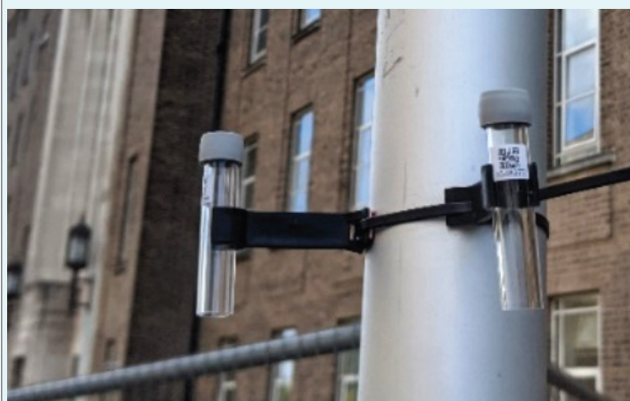
Fig 3. An example of diffusion tubes installed at Queen Elizabeth Hospital, Birmingham
