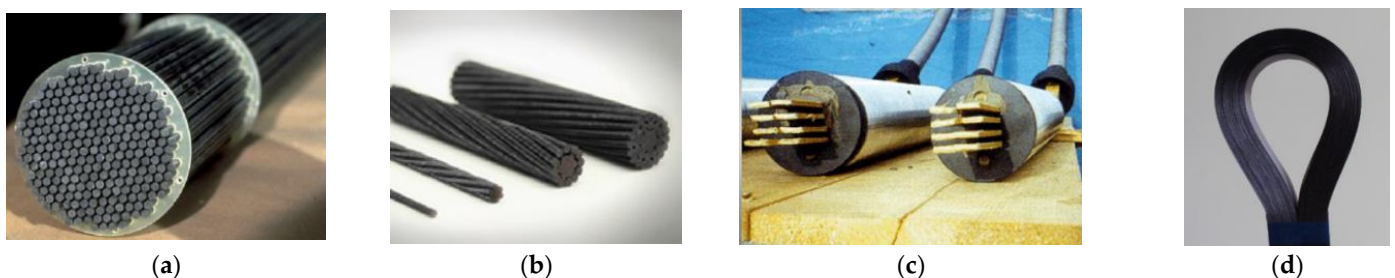
Figure 37. Types of FRP cables [30,31]: (a) FRP parallel wire cable; (b) FRP twisted wire cable; (c) FRP plate cable; (d) FRP sheet cable.
