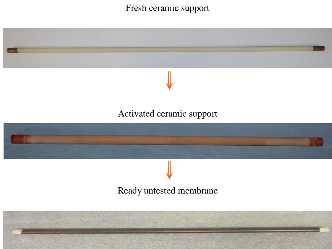
Figure 3.18 Pictorial views showing the fabrication of a membrane (from a fresh ceramic support to metallic composite membrane).
