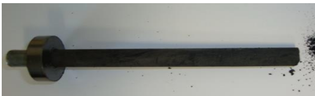
Figure A1. 8 Shows pictorial view for membrane HCME6001 that proves the presences of traces of carbon (coking).
