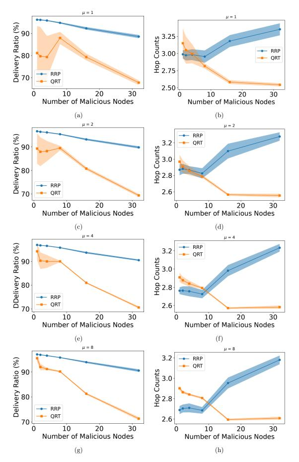
Figure 4.8: The average delivery ratio and hop counts under On-Off attacks for variable traffic rates
