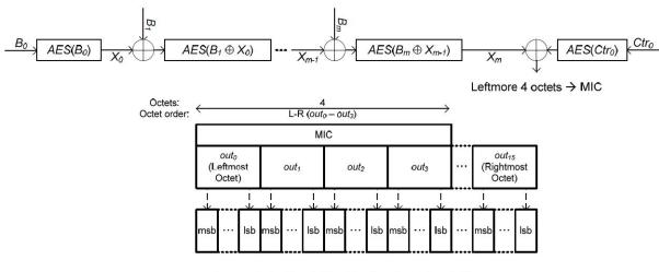
Figure 2.6: MIC calculation and transmit order [1]
