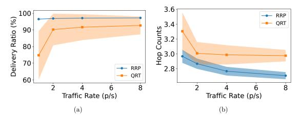
Figure 4.4: The average delivery ratio and hop counts under normal operation
