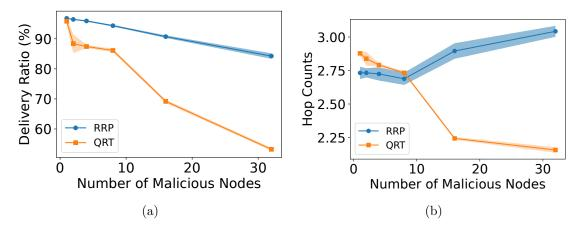
Figure 4.5: The average delivery ratio and hop counts under blackhole attacks
