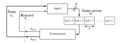
Figure 4.3: Graphical representation of the proposed RL model
