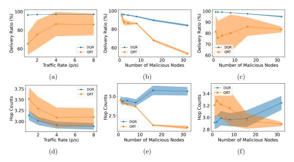
Figure 5.2: The average delivery and hop counts ratios under different conditions
