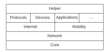
• Helper API contains classes and methods that provide high-level wrappers to encapsulate low-level API calls. It is widely used when scripting a simulation scenario.
