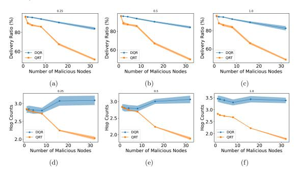
Figure 5.3: The average delivery and hop counts ratios under sinkhole attack
