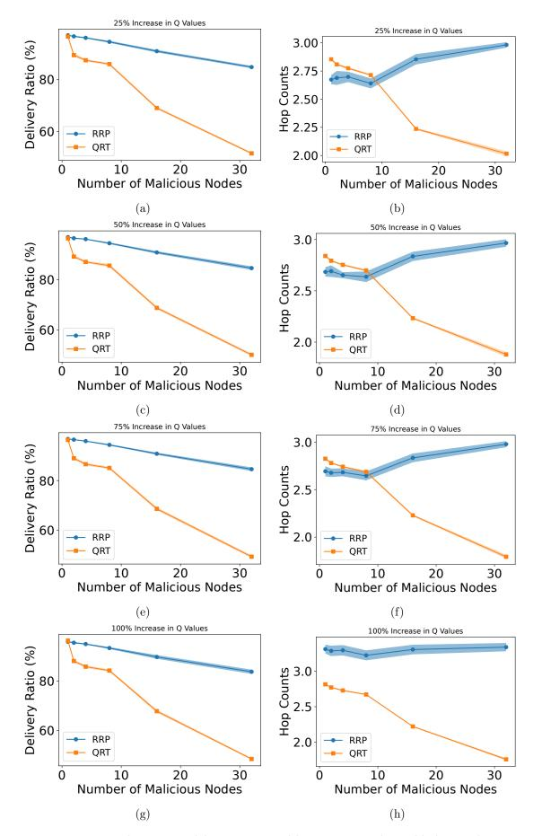
Figure 4.7: The average delivery ratio and hop counts under sinkhole attacks
