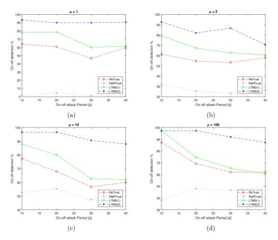
Figure 3.6: The detection performance for variable traffic rates
