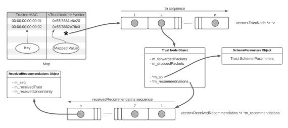
Figure 6.5: Trust Module Data Structure
