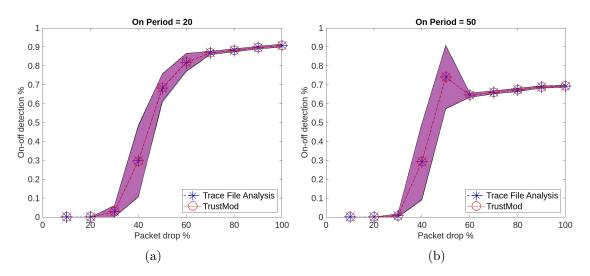
Figure 6.8: The detection performance for variable drop rates
