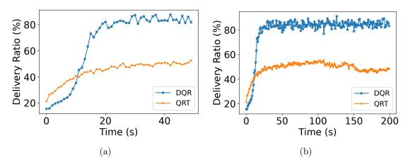
Figure 5.4: The average convergence time at the beginning of the simulation is shown in 5.4a, while in 5.4b the average delivery ratio is shown when three patients change their locations inside the ward at 100s and 150s
