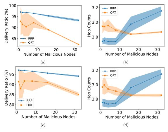
Figure 4.6: The average delivery ratio and hop counts under selective forwarding attacks
