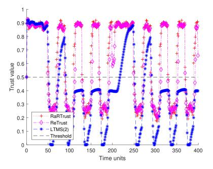
Figure 3.5: Trust evaluation for on-body and off-body SNs where the on-off attack starts at 50s and re-occurs again at 250s
