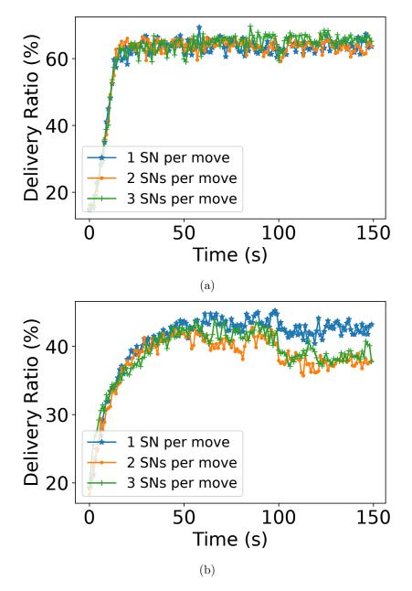
Figure 4.12: The average delivery ratio under different mobility scenarios for RRP and QRT, respectively
