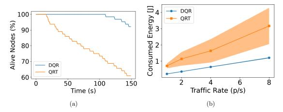
Figure 5.5: The average alive SNs ratio is shown in 5.5a, while the average consumed energy for variable traffic rates is shown in 5.5b
