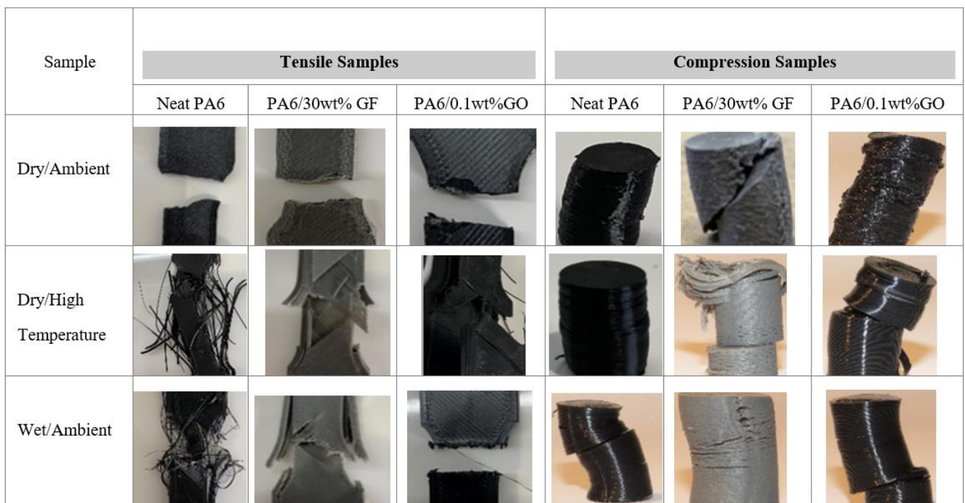
Figure 8. Damage features for tested samples (13 mm initial width for tensile samples and 12.7 mm initial diameter for compression samples).
