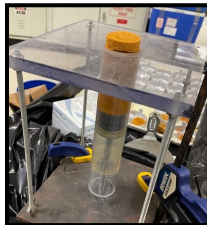
Figure 4 Sediment core extruder used to section sediment columns into ~ 1 cm intervals
