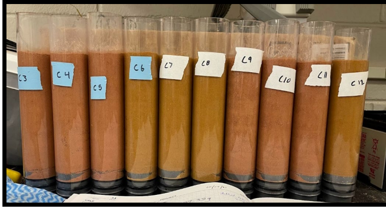
Figure 1 Sandy clay loam (SCL) and sand packed columns ( d \approx 14 cm) used in column flow experiments. Columns are pictured prior to exposure to wet-drying event.
