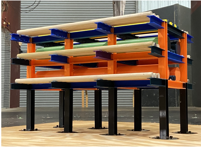
Figure 4.18: Pipe rack model at 30° angle
