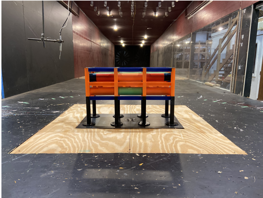
Figure 4.2: Test setup for pipe rack's force balance test
