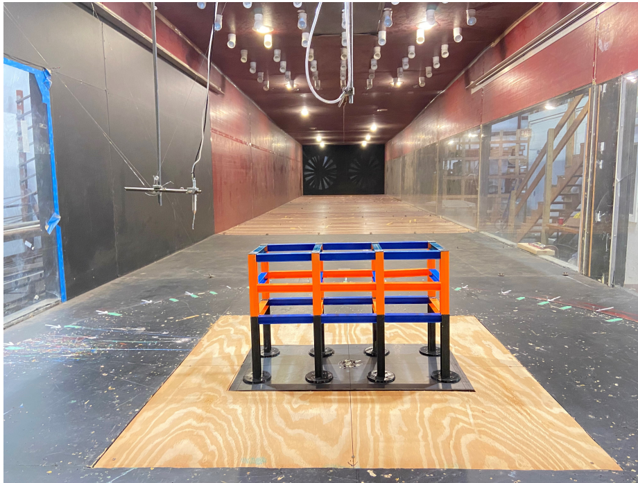
Figure 4.4: Bare frame of pipe rack
