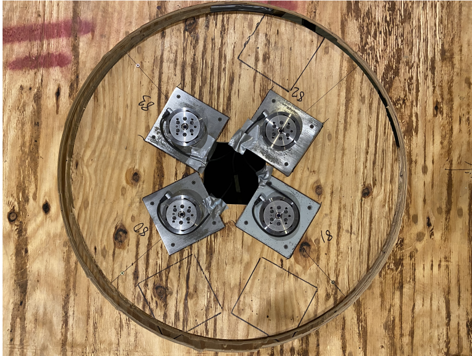
Figure 5.4: Load cells used to measure base shear of the attached columns
