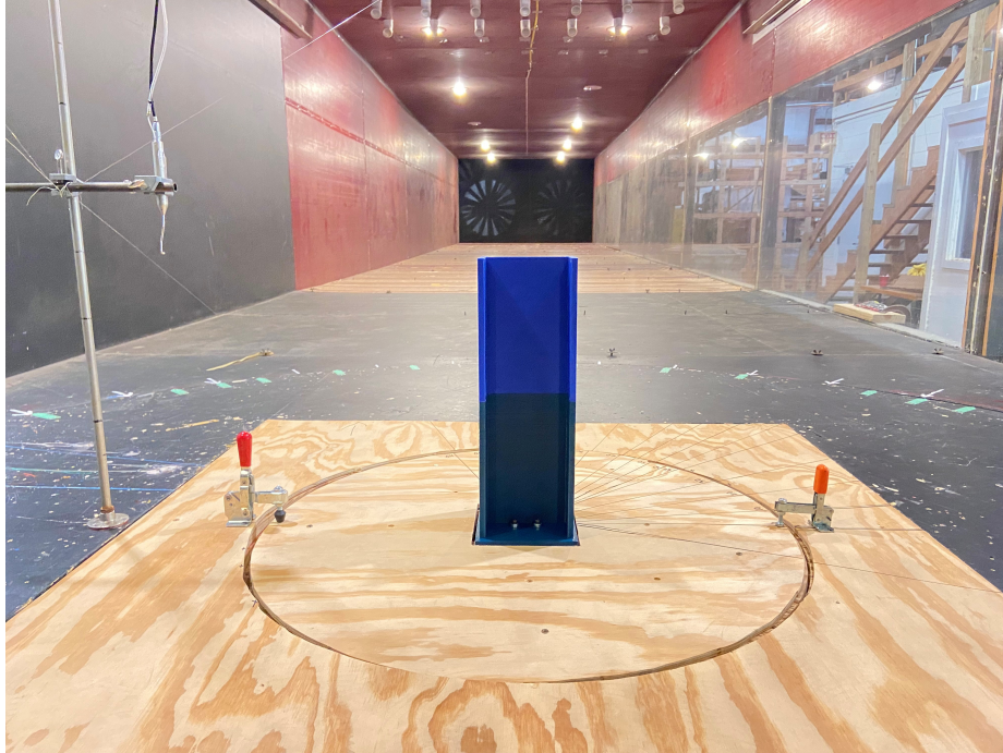
Figure 3.1: Experimental setup for wide flange section
