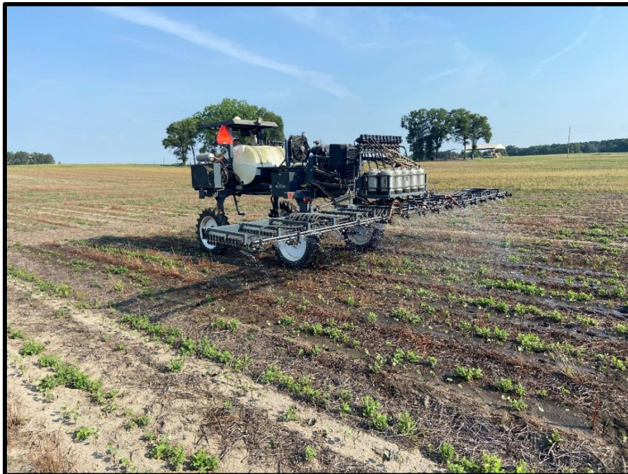
Figure 3.2. Image of MudMaster plot sprayer simulating rainfall after the insecticide application in the thrips study
