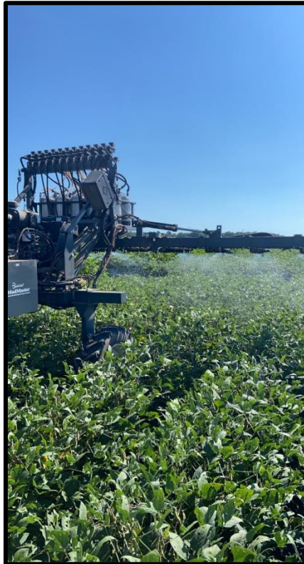
Figure 3.4. Image of MudMaster plot sprayer simulating rainfall in the soybean washoff study.
