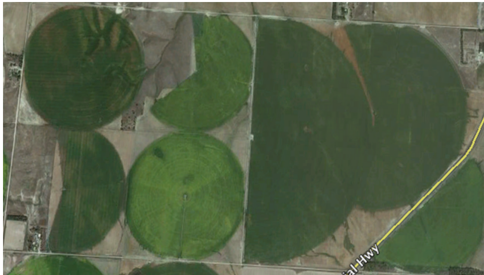
Figure 3. Example of the mix of partial-circle and full-circle center pivots used in South Carolina.
