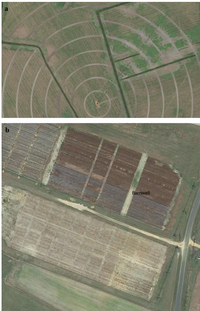
Figure 1. Counting the number of towers and distance between each tower in the (a) center pivot and (b) lateral move irrigation systems using the 2022 Google satellite image.
