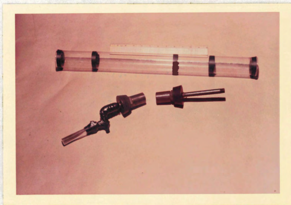
Figure 7. The electrodes, needle valve, and irradiation chamber.
