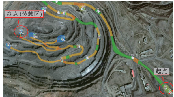
图 6 某露天矿区云平台显示的无人驾驶车辆行驶路径 Fig.6 Driving path of an autonomous vehicle displayed on the cloud platform in an open-pit mine
