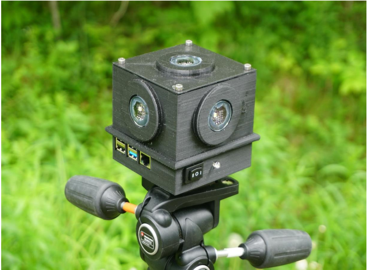
Figure 1. The LANcube v2 radiometer. On the bottom of the left face, are the USB and ethernet ports and on the right face one can see the operating switch and status RGB LED. At the center of each face lies a light color sensor (TCS 34725) that can measure both irradiances and illuminance. The size of the LANcube v2 is 9x9x9 cm.
