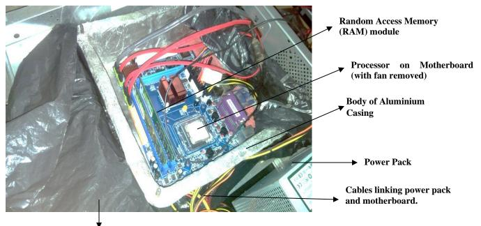
Plastic Casing realized via flexible plastic wrapping.
