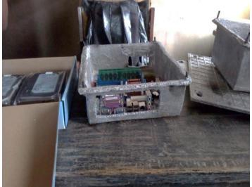
Figure 4 – Motherboard in Aluminium casing showing opening on casing side. The opening provides pathway and passage for connecting signal cable.
