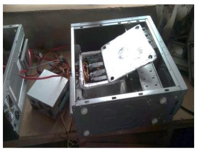
Figure 5 – Hard Disk Drives in Aluminium casing (with slanted lid) showing connecting cables to the motherboard in the next AT
