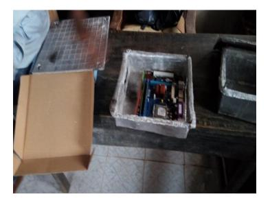
Figure 3 – Motherboard being placed in Aluminium casing.
