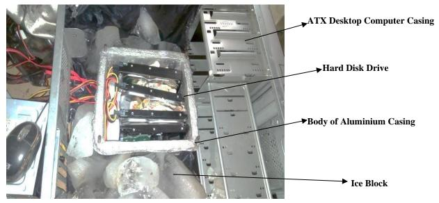
Figure 8 – Hard disk drives in Aluminium casing being cooled by ice blocks with connecting cables for signal transmission.
