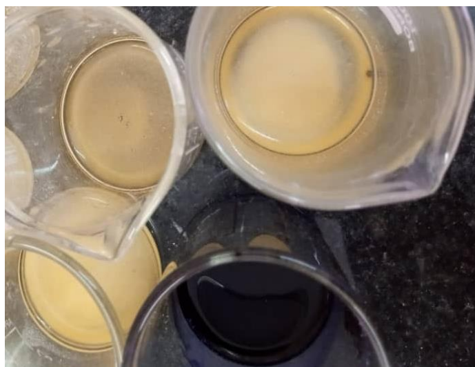
Figure 1a: Appearance of cellulose and starch in iodine solution
