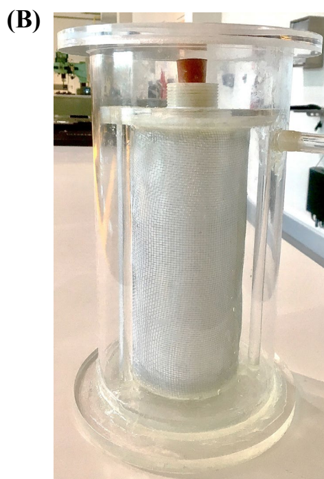
Figure 8: Radial-flow MBR design. (A) Schematic diagram of the radial flow tubular MBR, and (B) photo of the assembled tubular MBR
