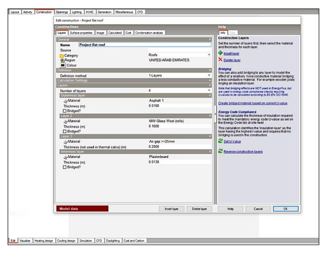
Figure C 7: Roof Construction Details
