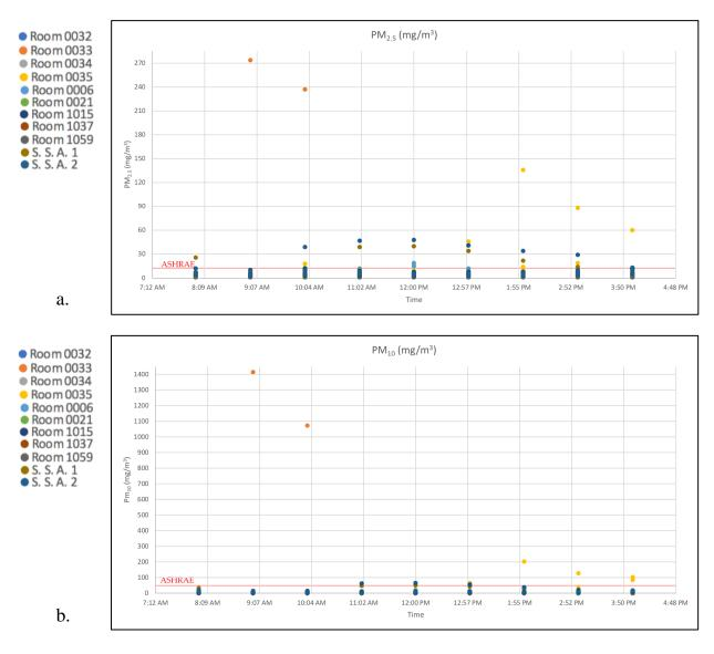
Figure 25: Hourly-Based Data For (a) PM2.5. (b) PM10
