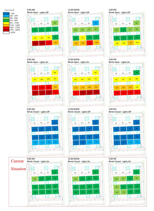
Figure 42: Lighting Levels Measurements for Classroom 1036 (First Floor)
