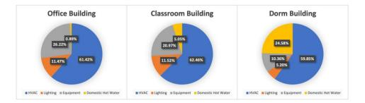
Figure 6: Baseline Energy Consumption Distribution by End Use. Source: (Al Amoodi A. & Azar E., 2018)
