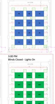
Figure 33: Lighting Levels Measurements for Classroom 0021 (Ground Floor)
