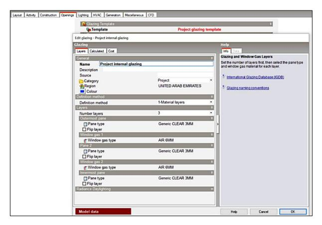
Figure C 10: Internal Glazing Details
