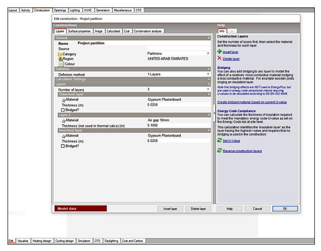
Figure C 6: Internal Partitions Construction Details
