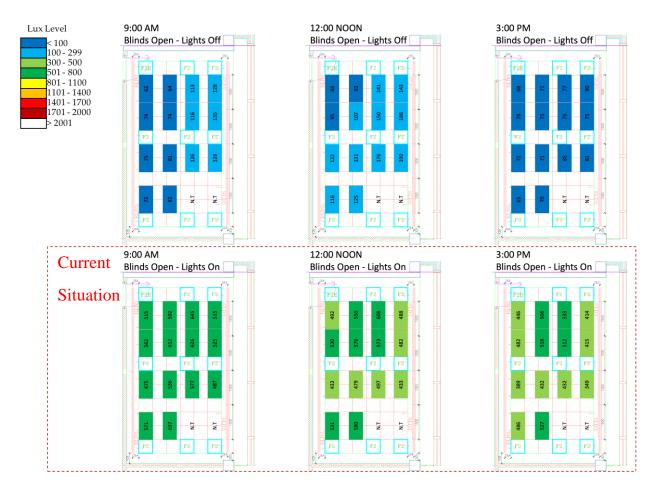
Figure 36: Lighting Levels Measurements for Classroom 1012 (First Floor)
