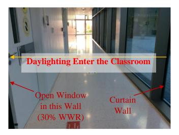
Figure 50: Daylight Comes from the Courtyard Can be Used in Classroom 0034
