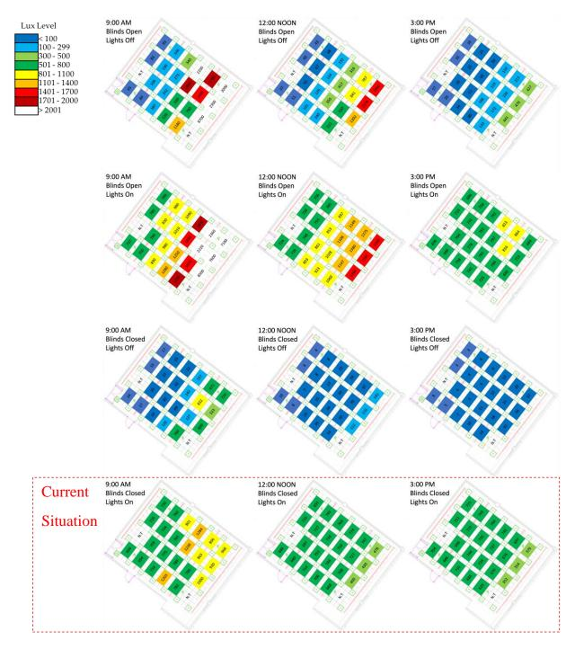
Figure 30: Lighting Levels Measurements for Classroom 0034 (Ground Floor)
