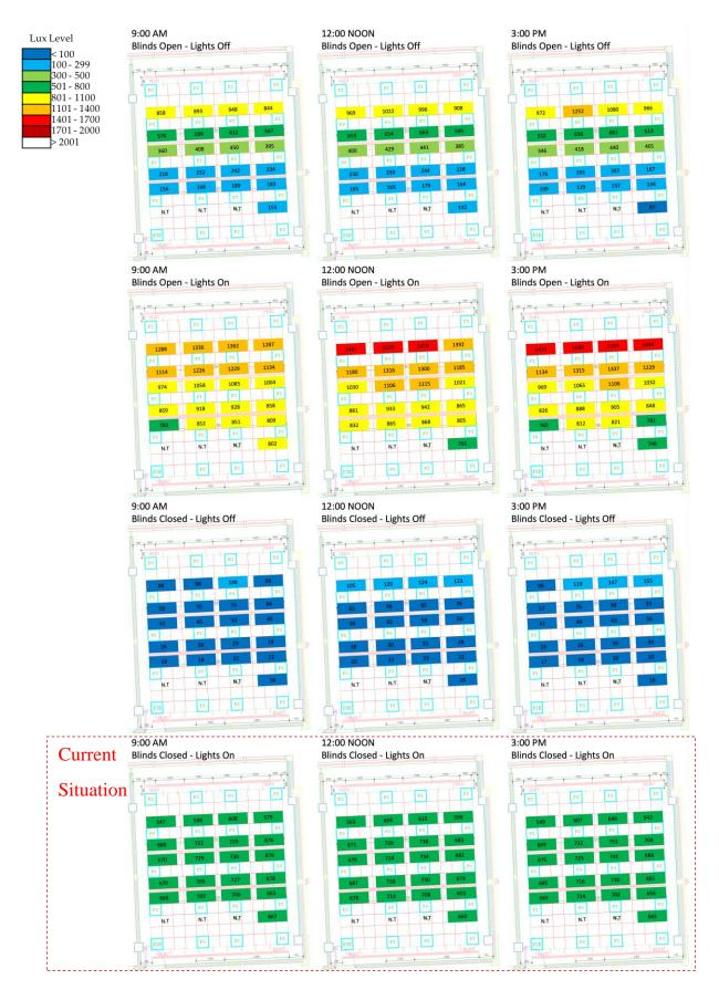
Figure 45: Lighting Levels Measurements for Classroom 1037 (First Floor)
