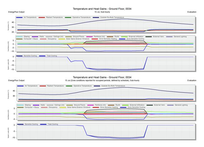
Figure 47: Cooling Load Graphs from DesignBuilder Software for Classroom 0034
