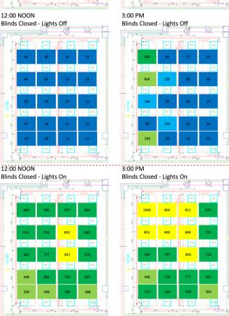
Figure 39: Lighting Levels Measurements for Classroom 1015 (First Floor)
