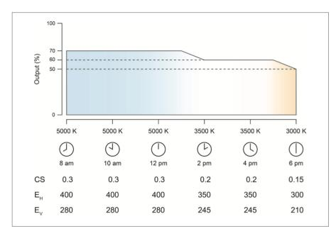
Figure 10: An Example of Customized CS Dosage Schedules. (EH) Horizontal Lux amount, (CS) Circadian Stimulus, and (EV) Vertical Lux. Source: (Figueiro et al., 2016)
