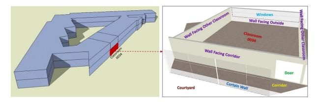
Figure 16: 3D Model and Classroom 0034 Created in DesignBuilder Software
