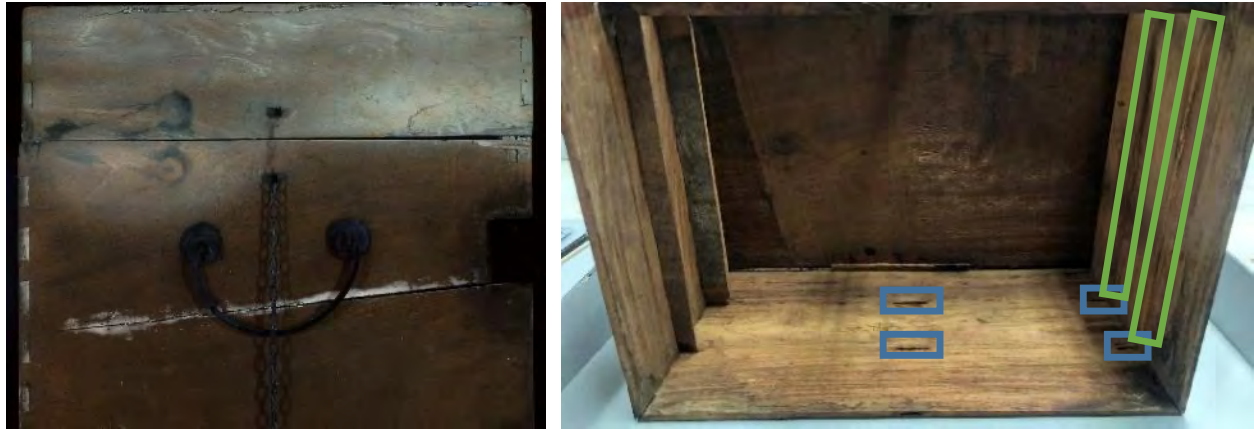
Fig. 5. Left: upper half of the left panel under UVA-induced visible fluorescence, highlighting the split running horizontally through the panel, and traces of a prior hinge attaching the lid. Right: Interior of the main cabinet, viewed from the underside. Adhesive glue lines from the missing side runners are outlined in green, and the hidden mortises for the runners are outlined in blue. The mortise for the base connection is also visible in the lower middle.
