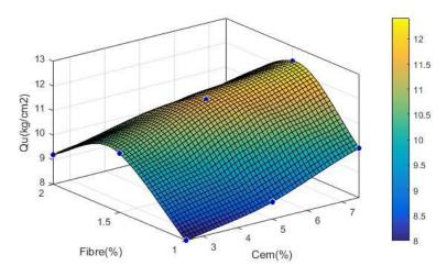
Fig. 6 - Investigation of the simultaneous effect of FN-fibers and cement on the compressive strength of modified sand soil
