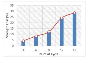
Fig. 10 - The effect of number of freezing-thawing cycle on the amount of strength loss
