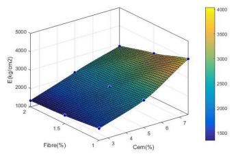
Fig. 9 - Investigation of the simultaneous effect of FN-fibers and cement on elasticity modulus
