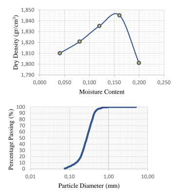
Fig. 1- Gradation curve(above), and compaction test results of the soil (below).
