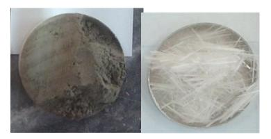
Fig. 3 - A view of the Portland cement type II (left), and FN-fiber (right)
