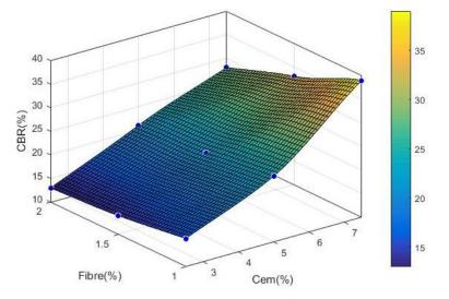
Fig. 8 - Investigation of the simultaneous effect of FN-fibers and cement on CBR
