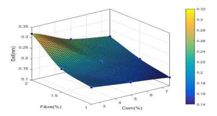
Fig. 7- Investigation of the simultaneous effect of FN-fibers and cement on soil deformation
