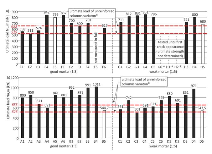
Fig. 5 - Comparison of experimentally determined ultimate strength in concentric compression of grouted brick columns with an artificial crack (a) and with an artificial cavity (b)
