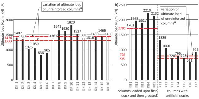
Fig. 5 - Comparison of experimentally determined ultimate strength in concentric compression of grouted stone columns with an artificial cavity (a) and with an artificial crack (b)
