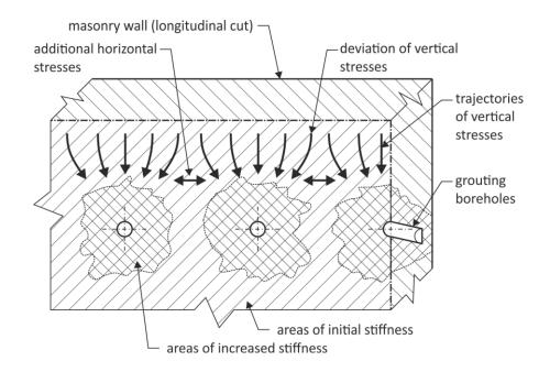
Fig. 1 - Increase of masonry stiffness due to the non-uniform penetration of the grout into the masonry structure
