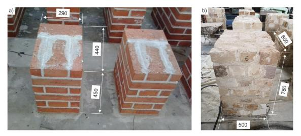
Fig. 3 Experimental specimens with aritificial crack and cavities; a) Brick masonry, b) Stone masonry
