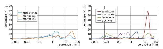
Fig. 4 - Distribution curves of pore representation in bricks and mortar (a) and stone masonry units (b)
