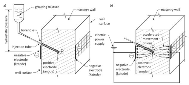
*Fig.* 2 - Combined electrophysical grouting of masonry structures; a) Grouting of masonry setup, b) Application of electrostatic field for propagation of grouting mixture through masonry
