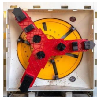
(a) Pipe jacking machine with three cutterheads (b) Pipe jacking machine with single cutterhead
