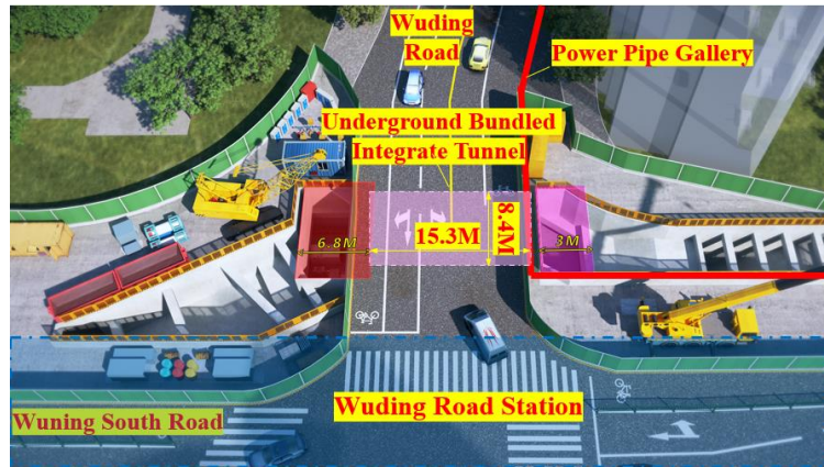
Fig.4-1 Plane graph of underground bundled integrate tunnel
