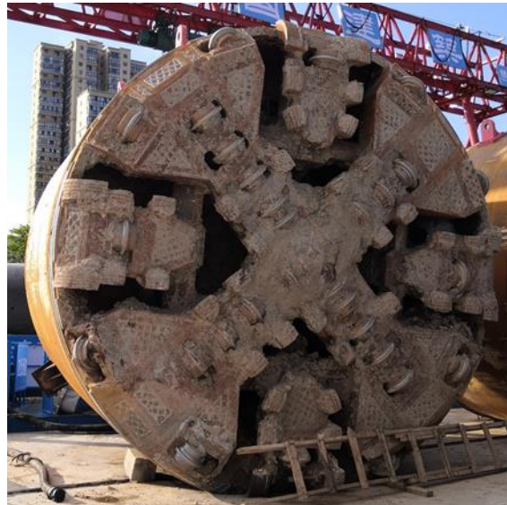
Fig. 3 – Pipe jacking machine
